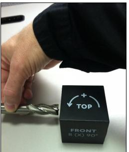
When using this training aid it is best to place the cube on a hard surface, and imagine that the tool is rotating around the part...don't rotate the cube.
